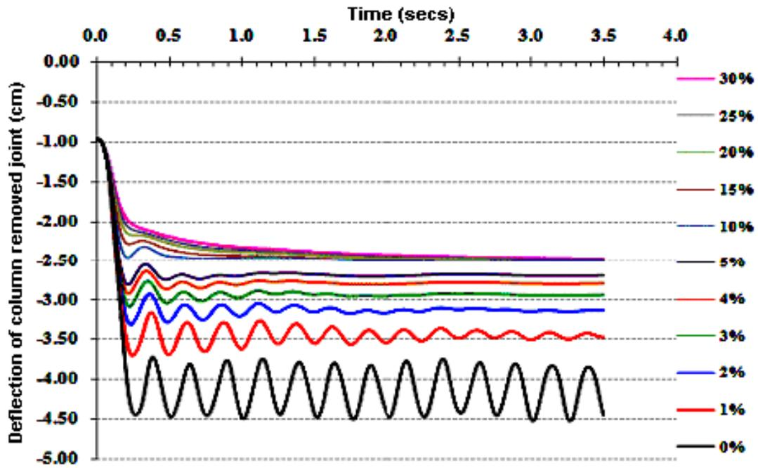
Fig. 13: Relationship between Damping Ratio and Deflection of Column Removed Joint at Grid 1D
