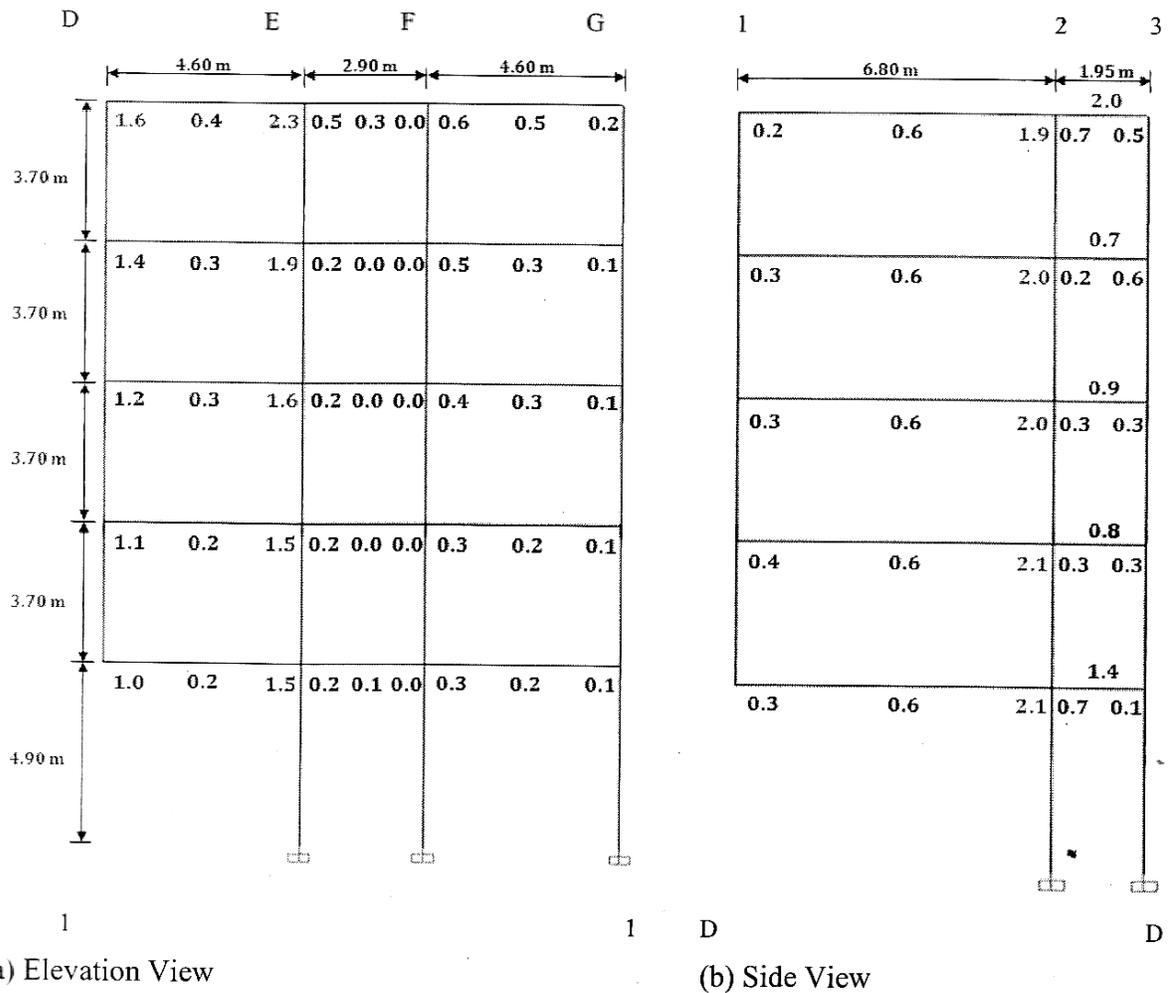
Fig. 6: DCR of Beams for Column Removal at Grid 1D of Block-1
