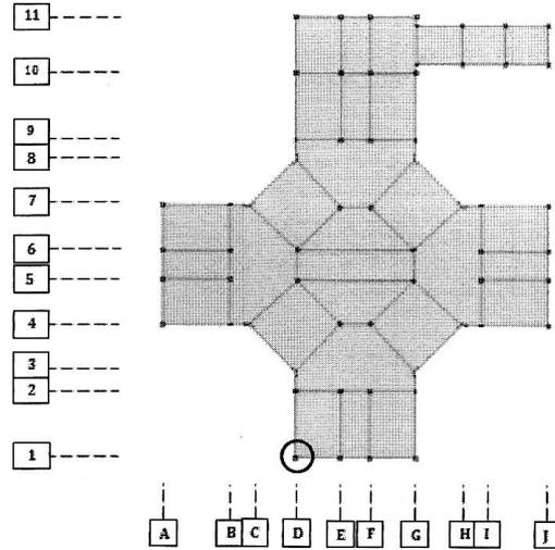
Fig. 5: Column Removal at Grid 1D of Block 1
