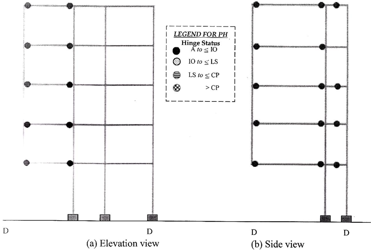
Fig. 9: Non-linear Plastic Hinges for Column Removal at Grid 1D of Block 1 under NLSA and NLDA
