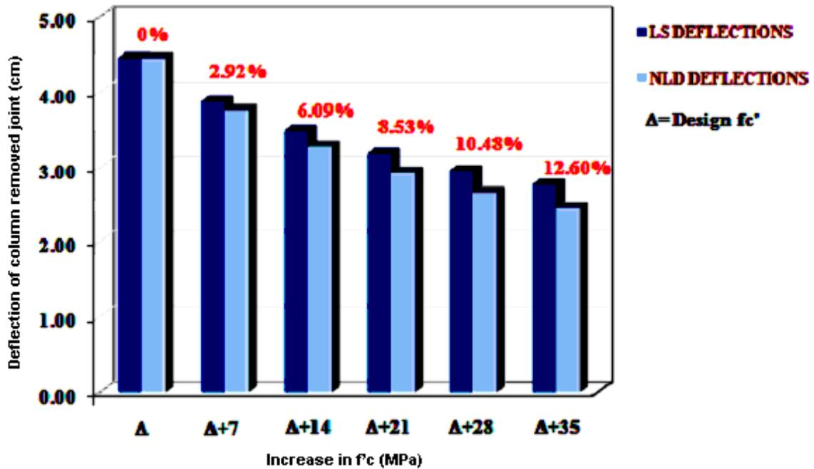
Fig. 12: Comparison of Linear Static and Non-linear Dynamic Deflections
