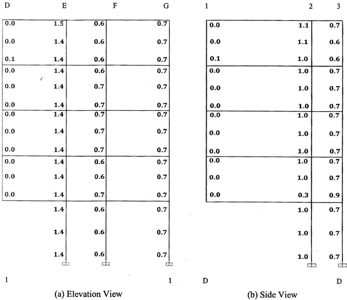
Fig. 7: DCR of Columns for Column Removal at Grid 1D of Block-1
