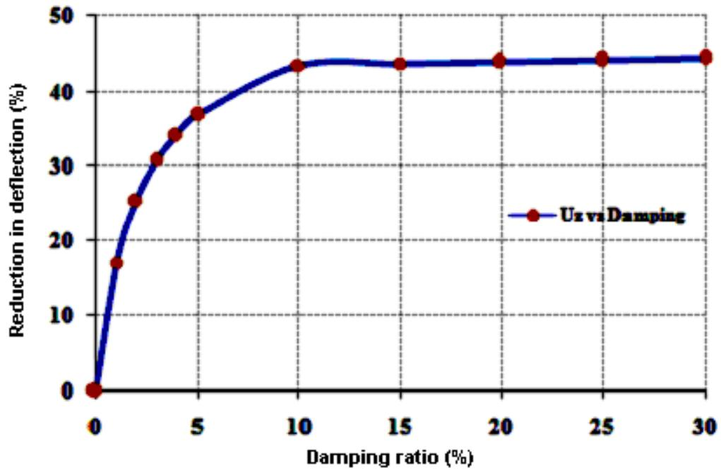
Fig. 14: Relationship between Damping Ratio and % Reduction in Deflection at Grid 1D
