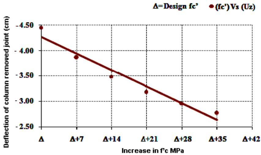
Fig. 10: Plot between  $f'c$  and Reduction of Deflection for Column Removal at Grid 1D
