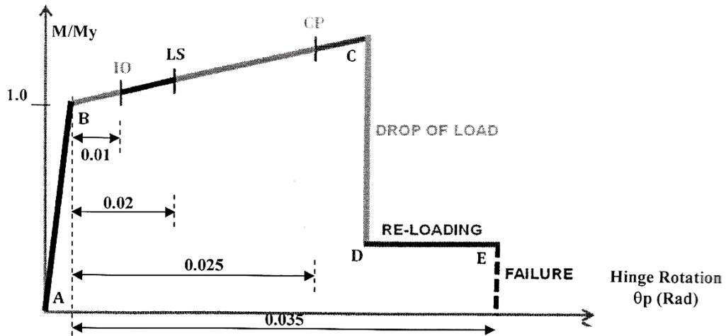
Fig. 8: Typical Plastic Hinge Backbone Curve
