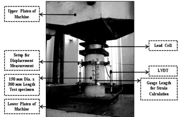
Fig. 2 Experimental Setup for E-value Test
