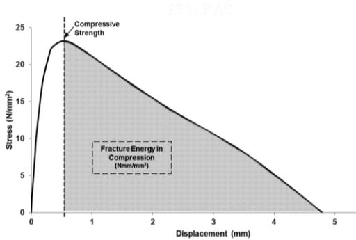
Fig. 3 Fracture Energy in Compression [12]
