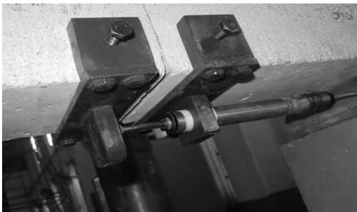
Fig. 6 Setup for CMOD Measurement
