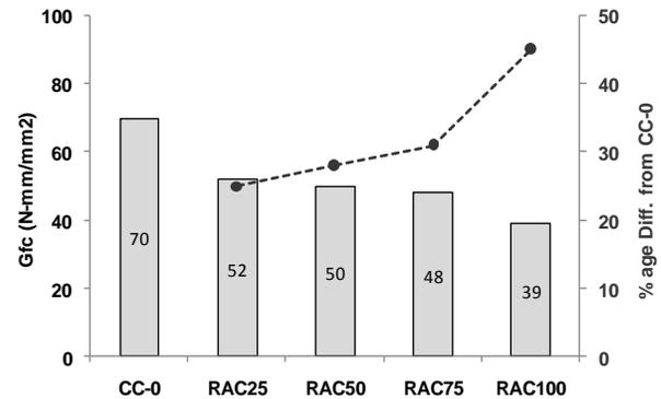
Fig. 10 Fracture Energy ( $G_{fc}$ ) in Compression
