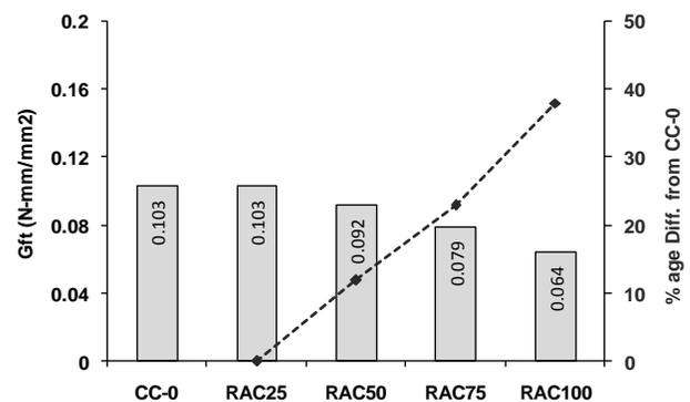
Fig. 11 Fracture Energy in Tension
