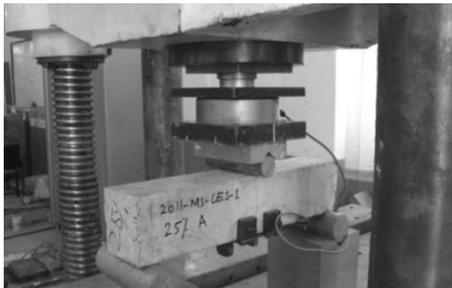
Fig. 4 Three Point Bending Testing Setup
