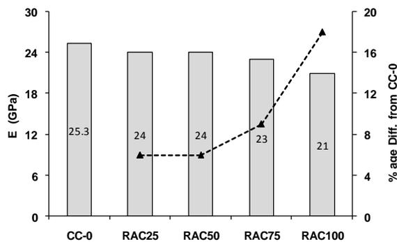
Fig. 9 Modulus of Elasticity
