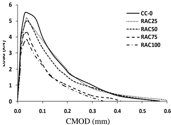
**Fig. 12** Load-CMOD Curve for Five Concrete Compositions
