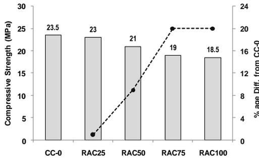
Fig. 8 Compressive Strength Of concrete
