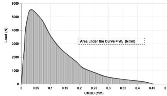
Fig. 7 Area under the Load-CMOD Curve for Fracture Energy in Tension
