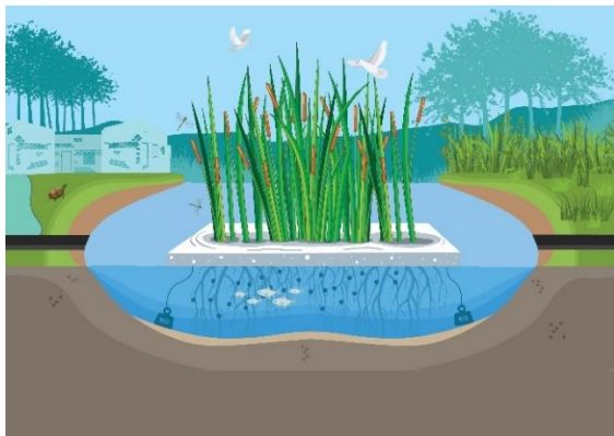
Fig. 2: Floating Treatment Wetland Design
