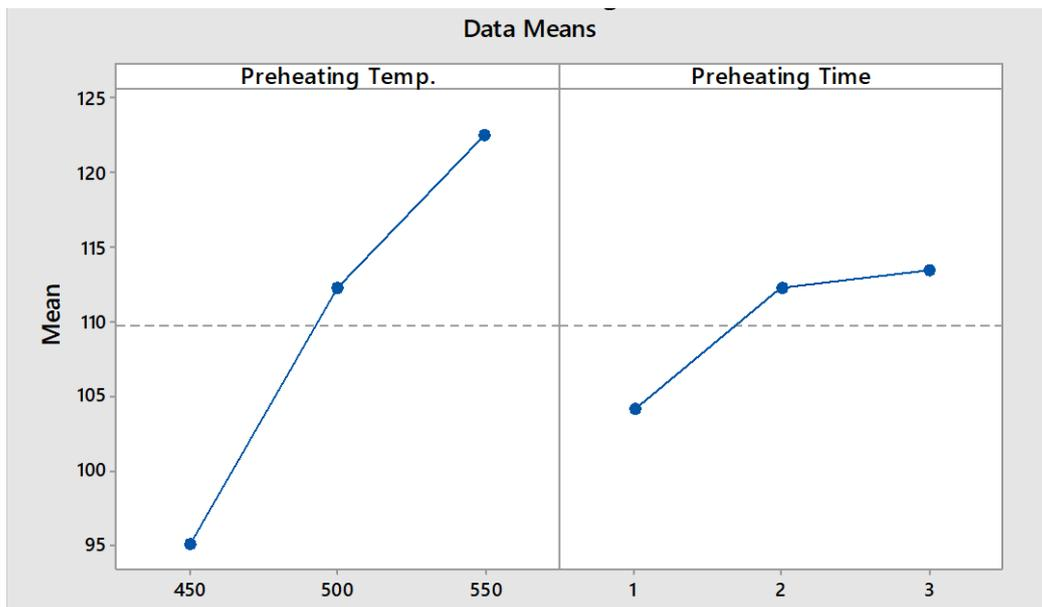
Fig. 3: Main effects plot of fatigue resistance
