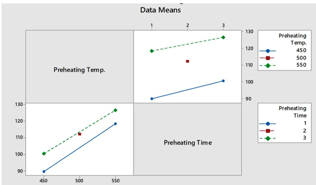
Fig. 4: Interaction plot of fatigue resistance
