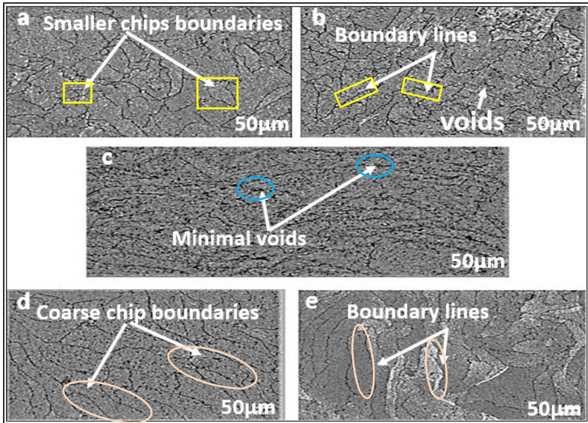
**Fig. 6:** Microstructure of extrudates at different PHT and PHti (a) 450°C and 1 hour (b) 450°C and 3 hours (c) 500°C and 2 hours (d) 550°C and 1 hour (e) 550°C and 3 hours
