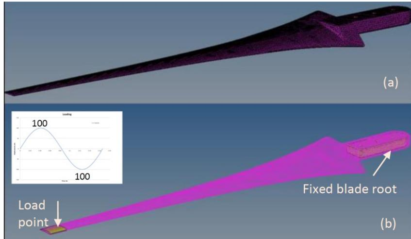
**Fig. 3:** FEMFAT images (a) Blade meshing, (b) Boundary conditions - fixed root and load point
