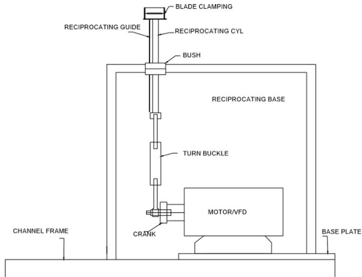
**Fig. 4:** Schematic of experimental set-up for fatigue testing
