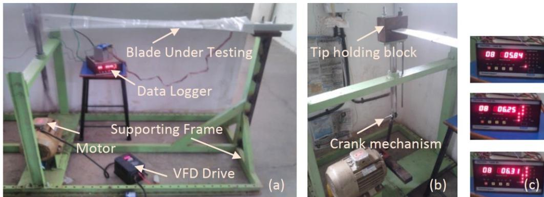
**Fig. 5:** The working experimental set-up for fatigue testing (a) Exploring blade motion and overall arrangement, (b) Exploring mechanism, (c) Dynamic data logger displays
