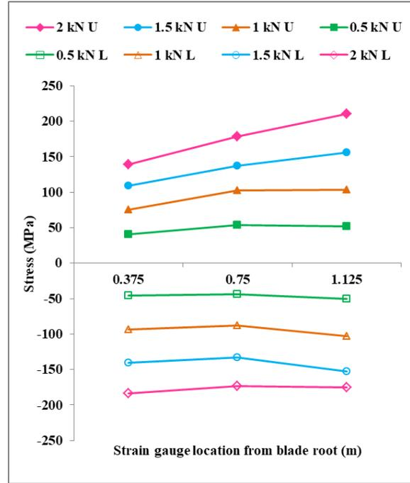
**Fig. 6:** Static stresses induced in the blade at different locations at various loads
