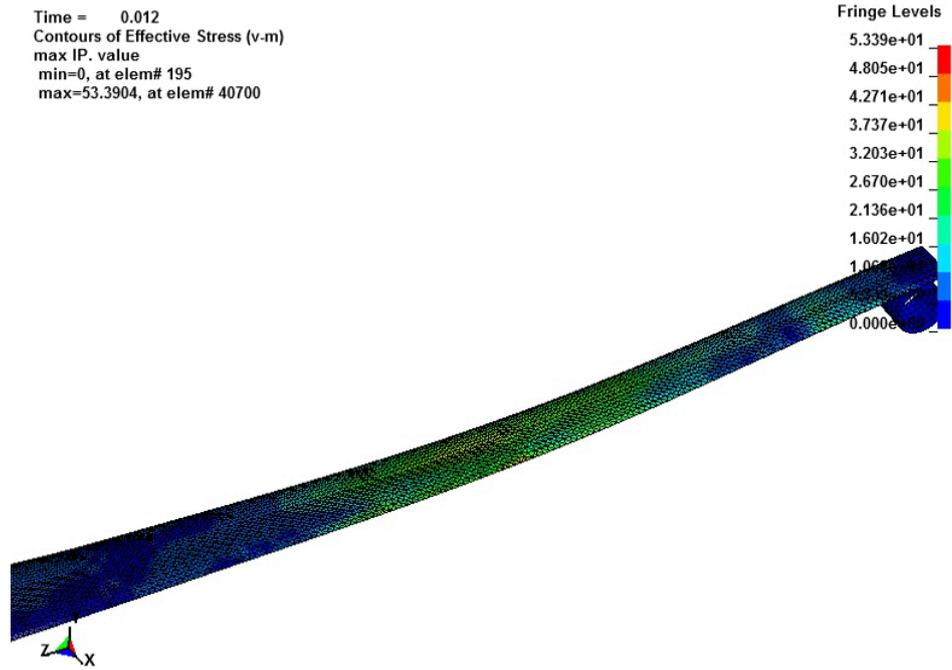
Fig. 7: A snapshot of FEMFAT showing the stresses during the cyclic loading
