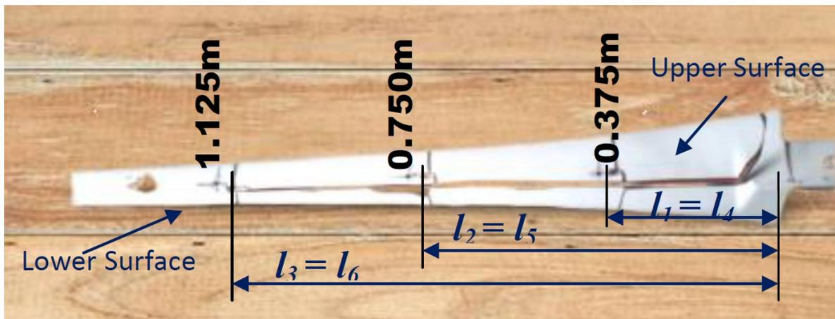
Fig. 2: Strain gauge locations on the blade from blade root
