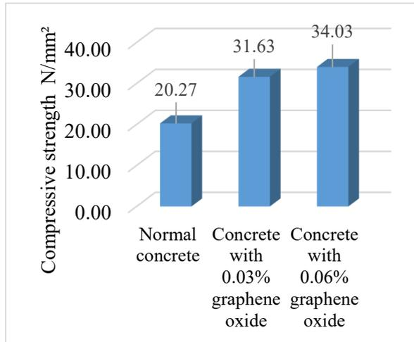
**Fig. 7:** Compressive strength of concrete specimens (with incorporation of 0 wt.%, 0.03 wt.% and 0.06 wt.% of GO)
