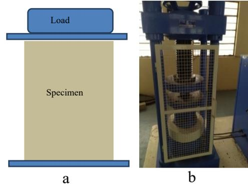
**Fig. 6: (a, b):** Schematic representation of measurement of compressive strength in concrete specimens
