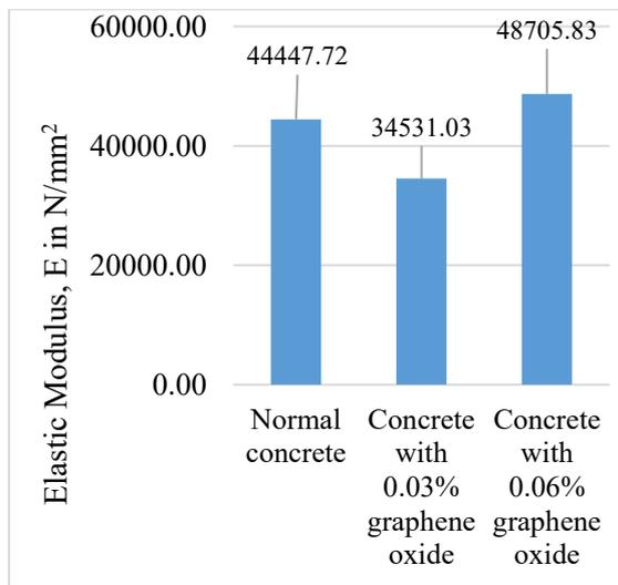
**Fig. 11:** Elastic modulus of concrete specimens (with GO)
