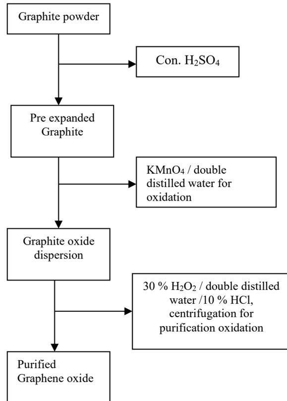
Fig. 1: Synthesis of Graphene oxide by Modified Hammer's method
