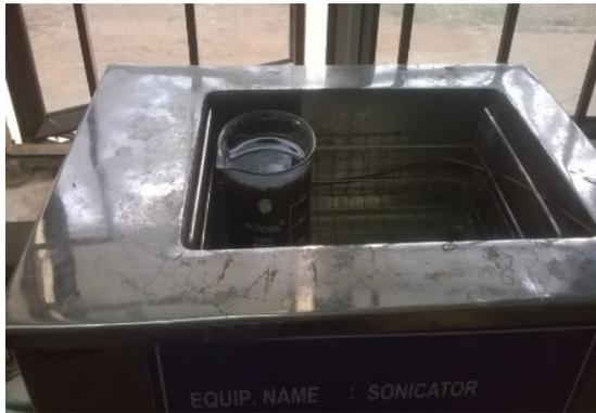
**Fig. 2:** Sonicator apparatus used for the exfoliation of GO powder in water
