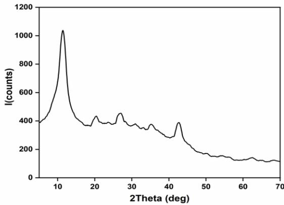
**Fig. 4:** XRD pattern obtained on GO nanostructured material prepared by Modified Hammer's method
