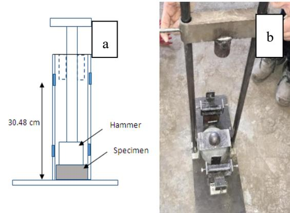
**Fig. 12: (a, b)** Schematic representation of measurement of ductility index in concrete specimens with impact testing machine.
