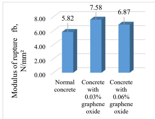
**Fig. 9:** Flexural strength of concrete specimens (with incorporation of 0 wt.%, 0.03 wt.% and 0.06 wt.% of GO)
