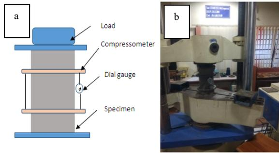
**Fig. 10: (a, b):** Schematic representation of measurement of elastic modulus in concrete specimens
