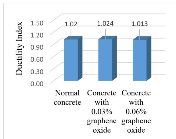
**Fig. 13:** Ductility index of concrete specimens (with incorporation of 0 wt.%, 0.03 wt.% and 0.06 wt.% of GO)
