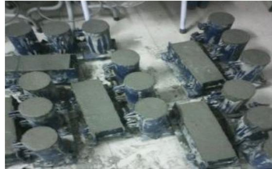
**Fig. 3:** The cast concrete specimens in different moulds
