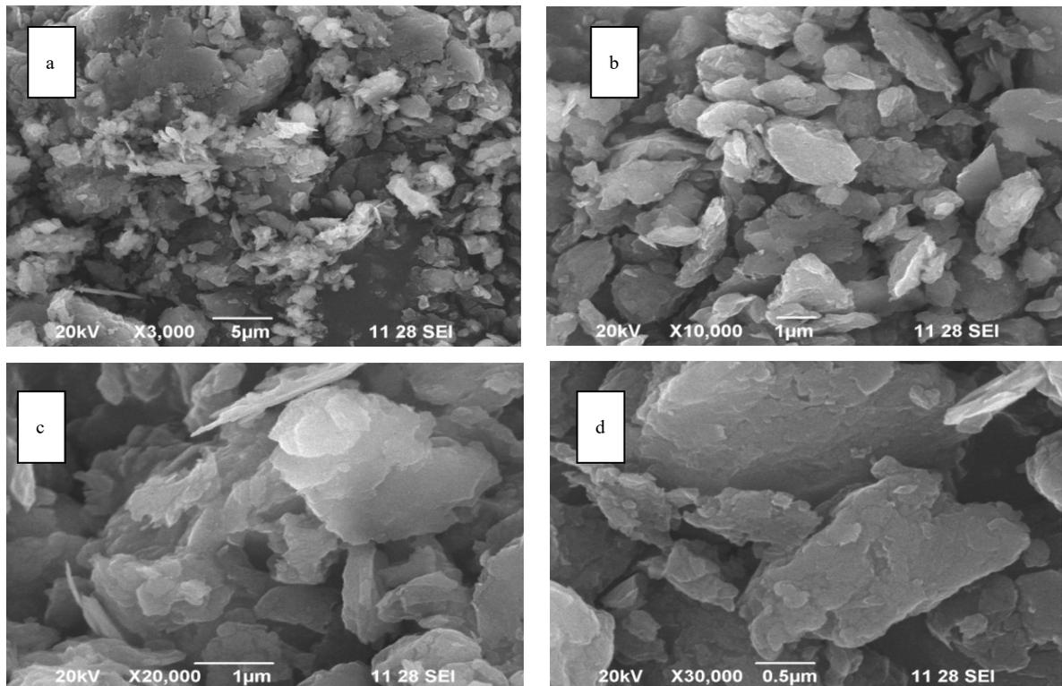
**Fig. 5:** SEM photographs obtained on GO nanostructured materials prepared by Modified Hammer's method (a) 3000x magnification, (b) 10000x magnification, (c) 20000x magnification, (d) 30000x magnification
