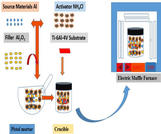
**Fig. 1:** Show the experimental procedure of Aluminide coating on Ti-6Al-4V alloy by Halide Activated Pack Cementation (HAPC)
