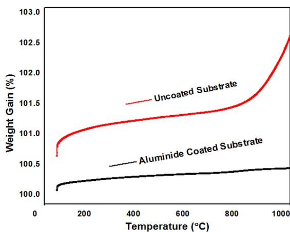
**Fig. 3:** Dynamic oxidation behavior of aluminide coating on titanium alloy (Ti-6Al-4V) for 3 hours
