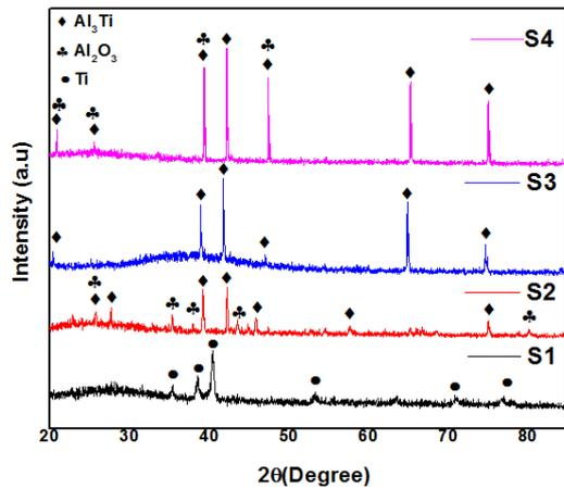
**Fig. 2:** XRD Analysis of Ti-6Al-4V alloy pack Aluminide (S1) Bare substrate (S2) Aluminide coating with residual powder for 3 hours (S3) Aluminide coating without residual powder for 3 hours (S4) Aluminide coating isothermal oxidized
