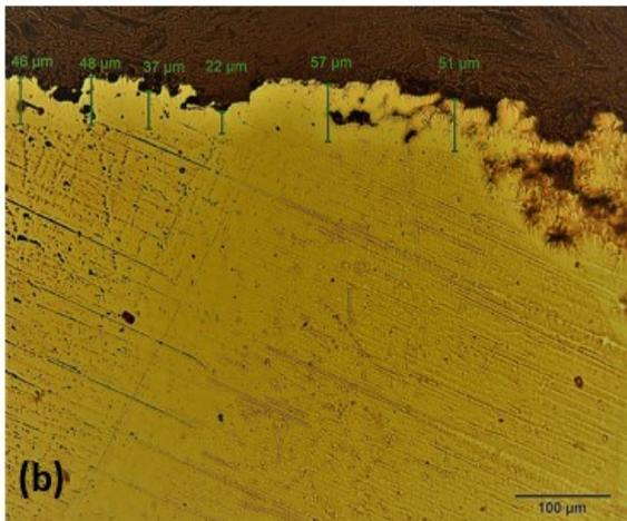
**Fig. 5:** The cross-sectional optical micrograph of aluminide coatings on titanium alloy Ti-6Al-4V for 3 hours (a) coated substrate (b) after oxidation
