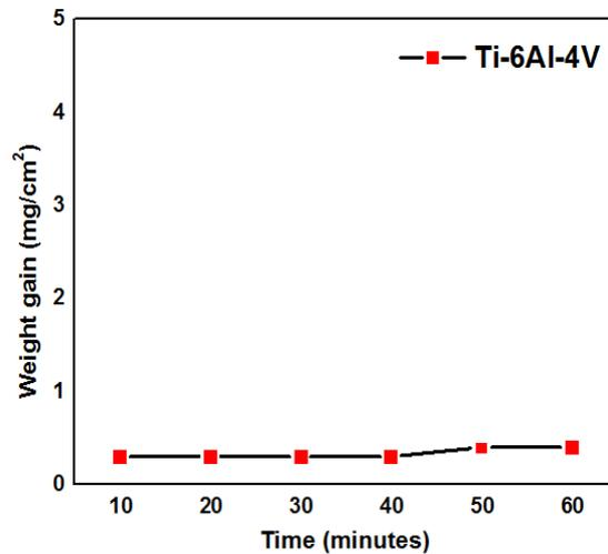
**Fig. 4:** Isothermal Oxidation of aluminide coated of titanium alloy (Ti-6Al-4V) for 3 hours
