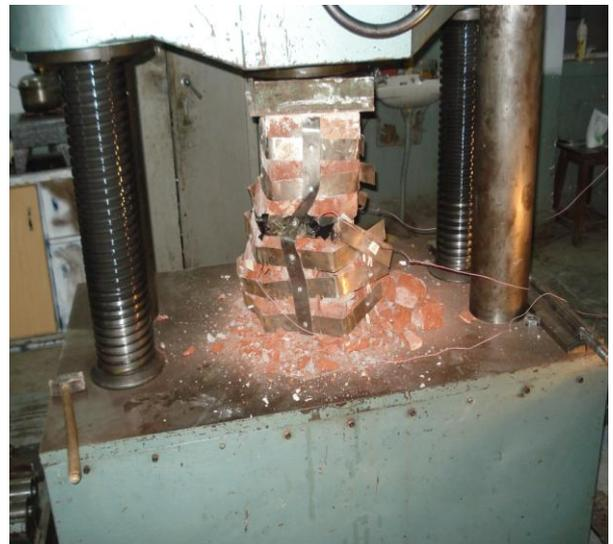
Fig.6a –Heavily reinforced column-10 at failure
