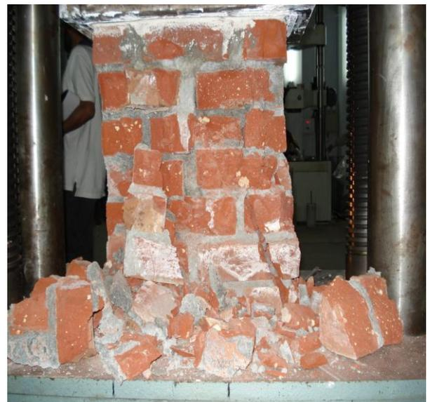
Fig.6b –Un-reinforced column-20 at failure
