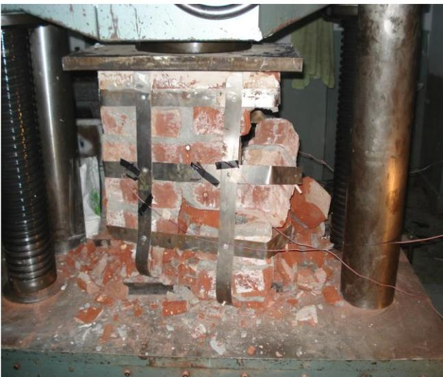
Fig 6d – Moderately reinforced col20 at failure
