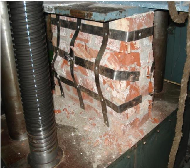
Fig 6c– Moderately reinforced col30 at failure
