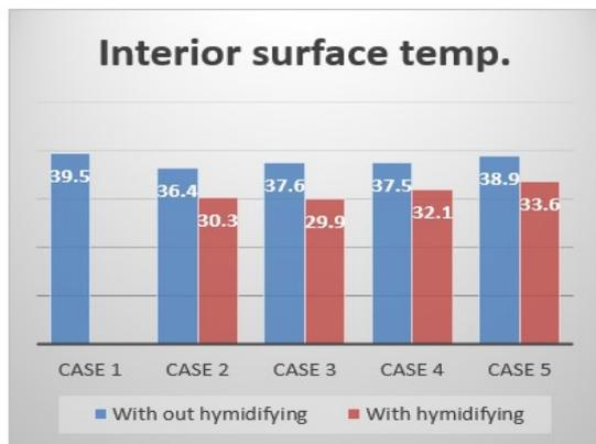
Fig. 8: Annual average for interior surface temperature for Studied walls (T<sub>i</sub>) with and without humidifying ambient air
