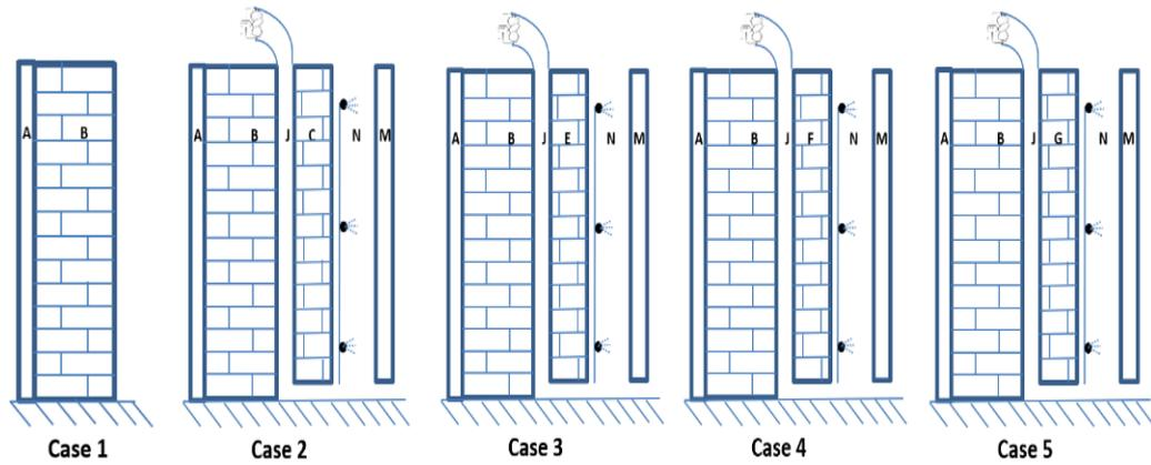
**Fig. 2:** Types of studied walls (A Gypsum 25 mm, B Common rick 240mm, C Face brick 120 mm, E Tile brick 40mm, F Limestone 40mm, G Solid cement brick 40mm, M Window screen / mesh, N External air gab and humidification System, J Ventilation duct 50mm)
