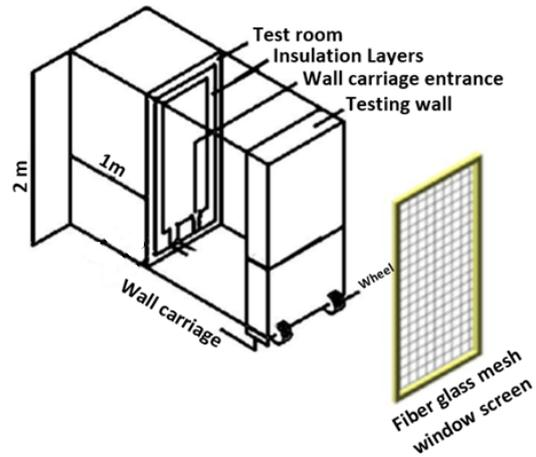
**Fig. 1:** Schematic illustrations the details of testing room
