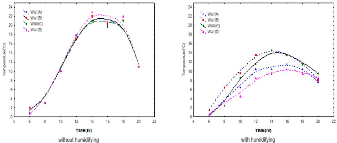
**Fig. 6:** Temperature differences between external and interior surface ( $\Delta T_{o-i}$ ) for all walls (To external surface temperature, Ti Interior surface temperature, Th Ambient air temperature)
