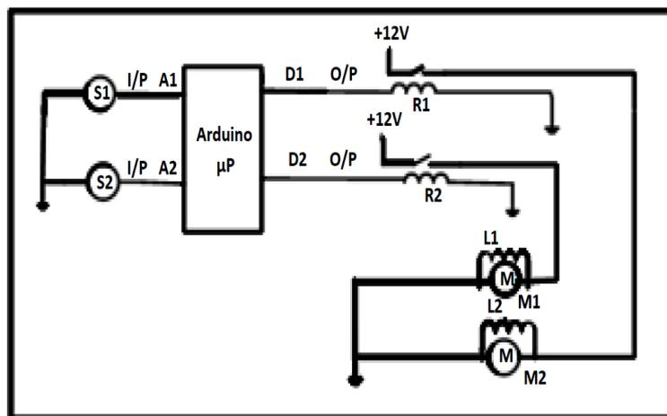
**Fig. 3:** Control circuit which used in humidifying ambient air (S1, S2 moisture sensors, R1, R2 water pumping relay and M1 water pump, M2 stand by pump)
