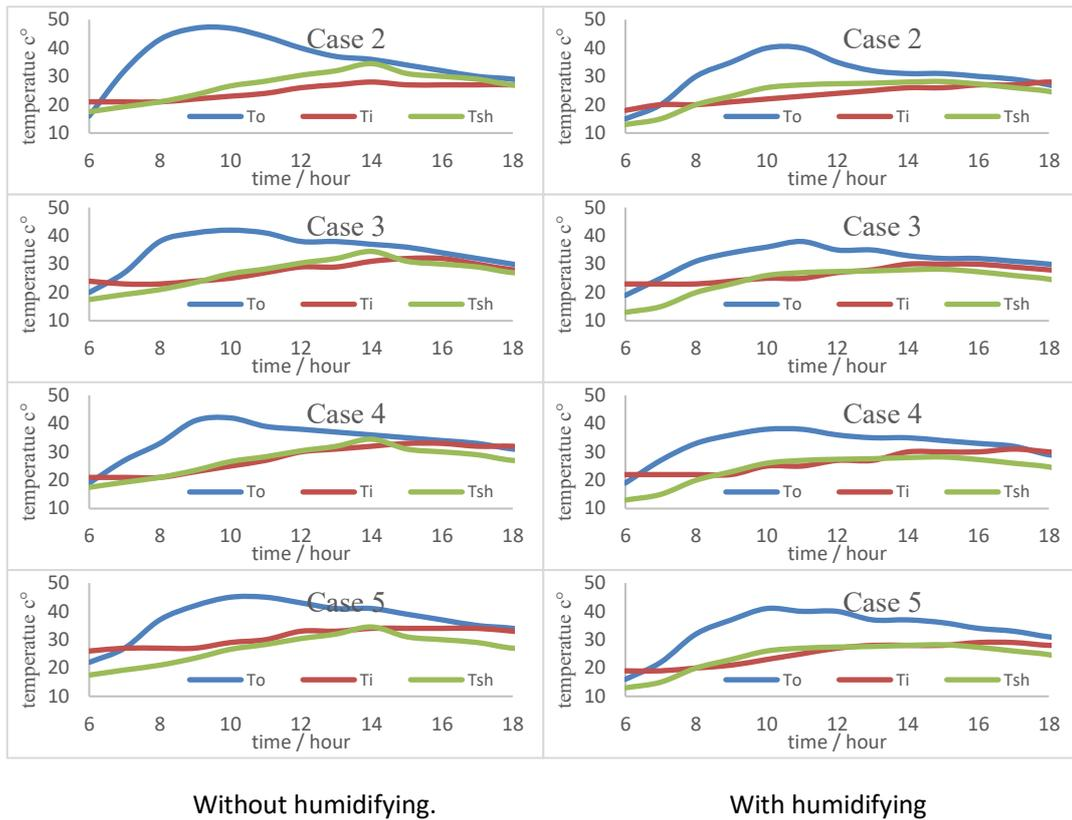
**Fig. 5:** Thermal behavior of Studied walls with and without humidifying ambient air (To external surface temperature, Ti Interior surface temperature, Tsh Ambient air temperature)
