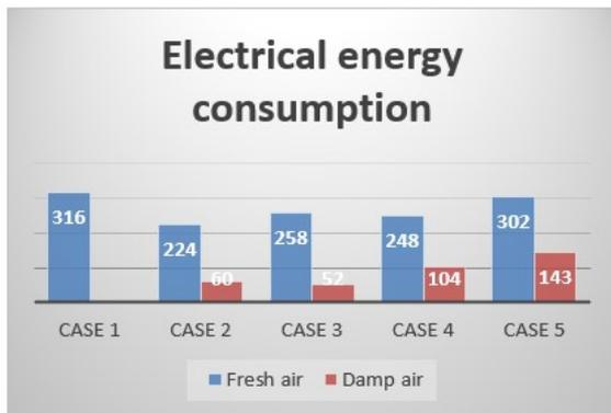
Fig. 9: Annual electrical energy consumption for cooling purposes with and without humidifying ambient air
