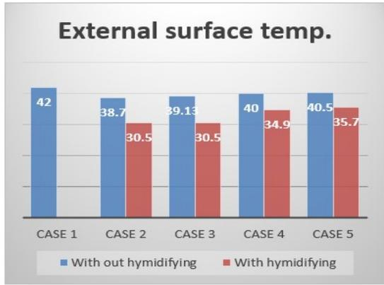
Fig. 7: Annual average for external surface temperature for Studied walls (T<sub>0</sub>), with and without humidifying ambient air
