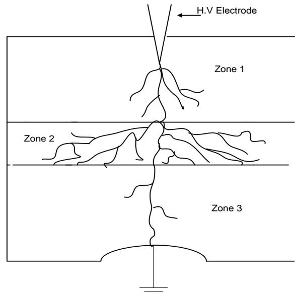
**Fig. 6b: Tree pattern in resin base specimens**
