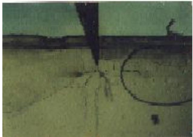
**Fig.10 Pattern of Tree growth in a specimen containing melinex barrier at  $45^{\circ}$**
