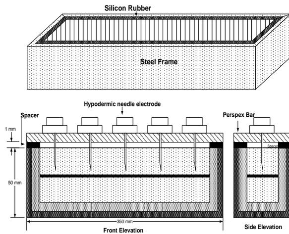
Fig. 2: Specimen manufacture method
