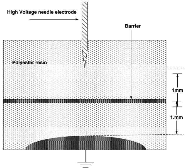
Fig. 4(a): Point plan Specimen containing barrier
