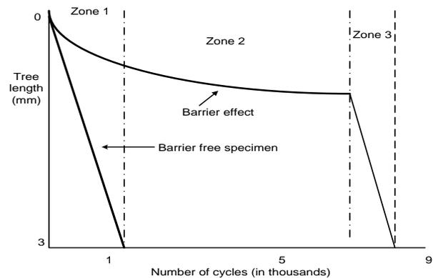
**Fig. 6a: Treeing in resin base specimens**
