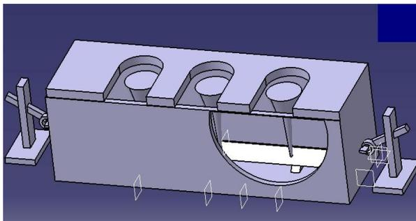
Fig. 3: Specimen manufacture method when barrier disposed at 45°
