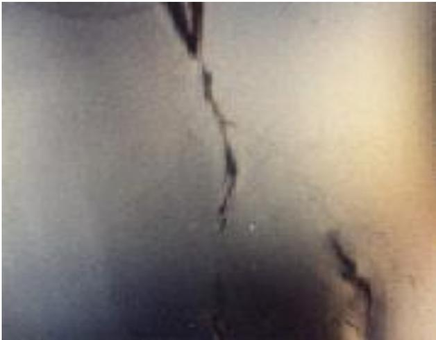
**Fig. 9: Tree growth in a specimen containing glass barrier at  $90^{\circ}$**
