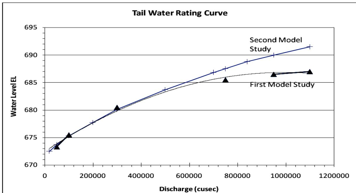
Fig. 1 Tail water rating curves employed in the model studies.
