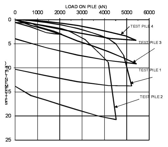
Figure 2: Load-settlement graphs for four pile load tests in clay.
