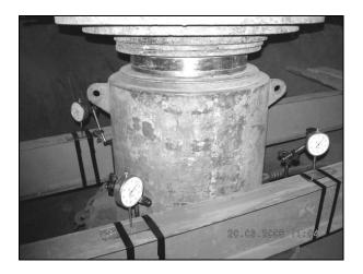
**Plate 2:** A view of the jack, settlement dial gauges, and reference beams used under the loading plat-form.
