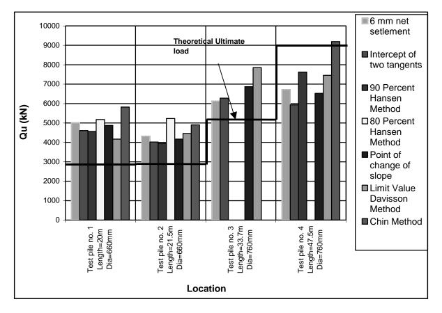
Figure 3: Ultimate loads using different methods.
