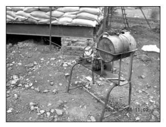
Plate 3: Oil reservoir pump and pressure gauge
