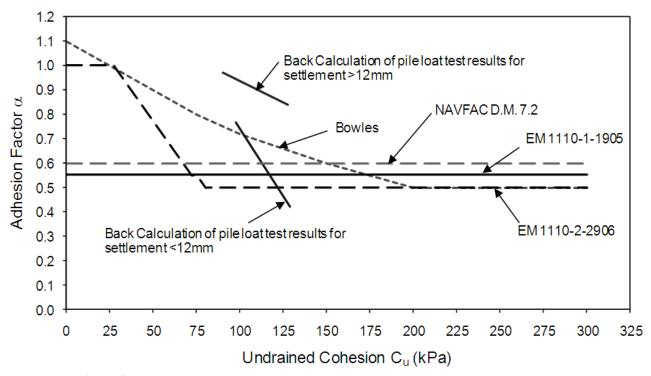
Figure 4: Relationship between adhesion factor  $\alpha$  and undrained cohesion C<sub>u</sub>. (From sources noted)
