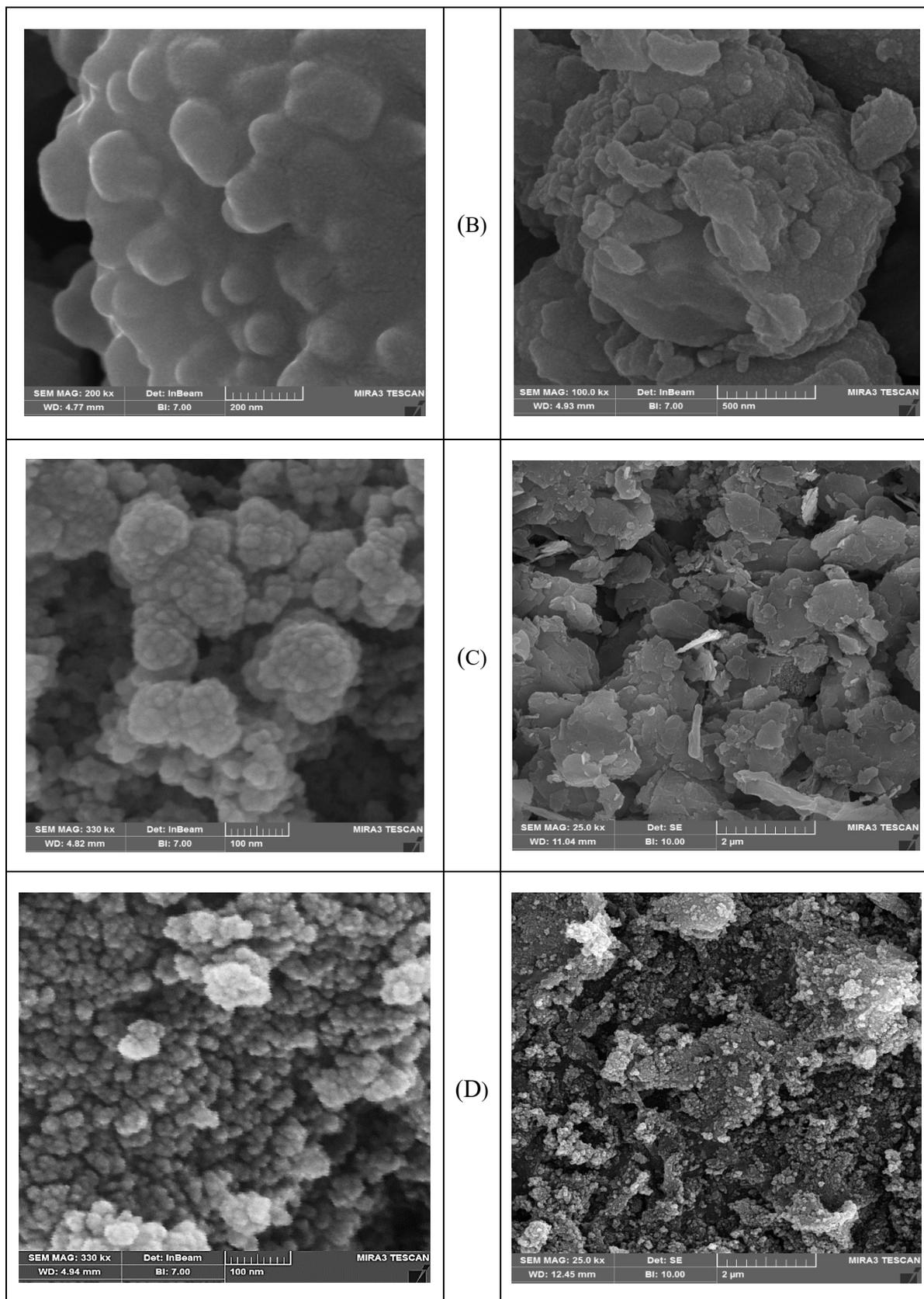
**Fig. 2:** SEM images of prepared nanoparticles for (A). ZnO, (B) Cu<sub>2</sub>O, (C) MgO and (D) TiO<sub>2</sub>
