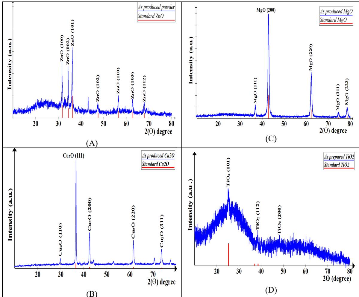
Fig.1: XRD patterns the powders of: A. ZnO, B.Cu<sub>2</sub>O, C. MgO and D. TiO<sub>2</sub>
