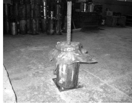
Figure 5: Pullout sample immediately after casting..
