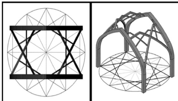
**Fig. 1:** Plan, three-dimensional model and components of Karbandy. Source: (Mansoor & seena, 1990, p. 99)
