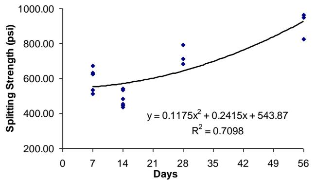
Fig.6 Overall split cylinder strength development trend.
