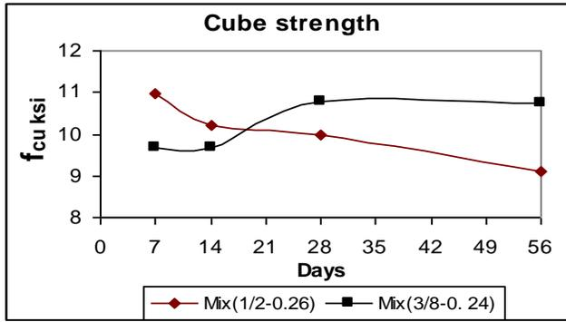
Fig.1 Cube strength comparison
