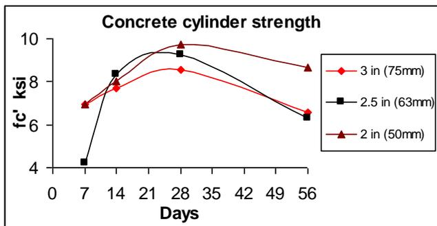
Fig. 3 Concrete cylinder strength
