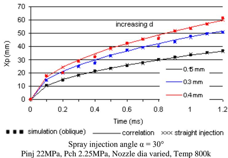
**Fig. 6: Spray Tip Penetration vs Time**
