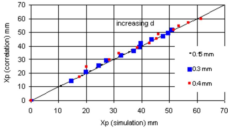
**Fig. 7: Penetration (correlation) vs Penetration (simulation)**
