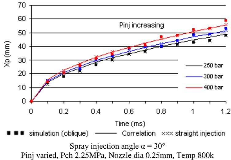
**Fig. 4: Spray Tip Penetration vs Time**
