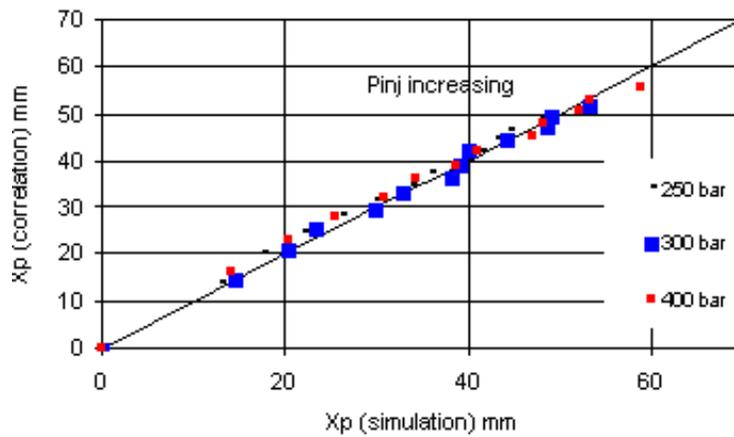
**Fig. 5: Penetration (correlation) vs Penetration (simulation)**
