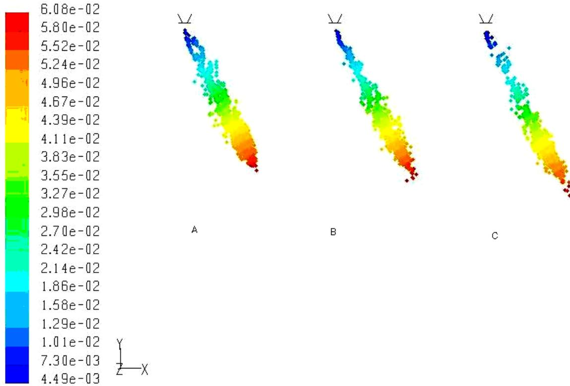
A=20, B= 40 and C=80 MPa Injection Pressure
