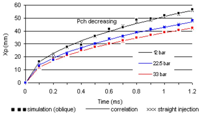
Spray injection angle  $\alpha = 30^\circ$
