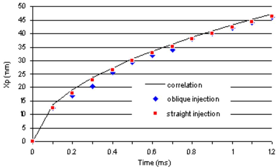
Fig. 3: Spray Tip Penetration vs Time, P<sub>ch</sub> 2.25MPa, P<sub>inj</sub> 22MPa, Nozzle dia 0.25mm, Temp 800k
