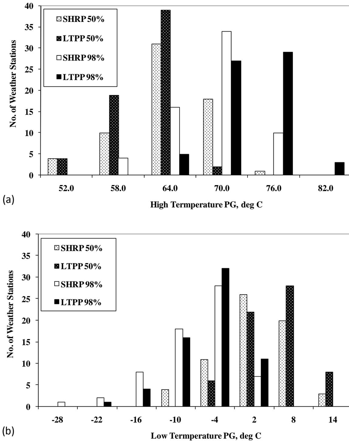
Figure 3 Histogram of High/Low Pavement Temperatures for 64 Stations
