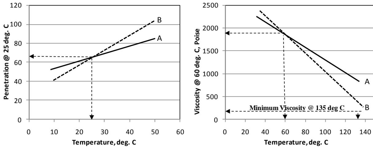
**Figure 1:** Graphical Comparison of two binders meeting Penetration and Viscosity Grading Specifications
