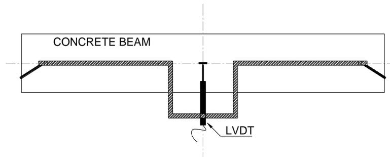
**Figure 5:** Deflection measurement scheme
