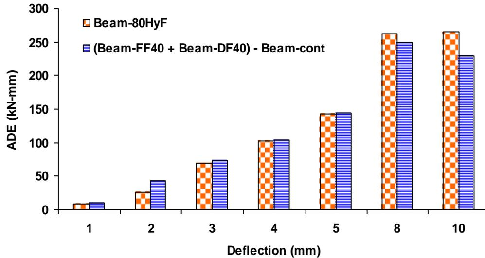
**Figure 11:** Synergy assessment for Beam-80HyF in terms of dissipated energy
