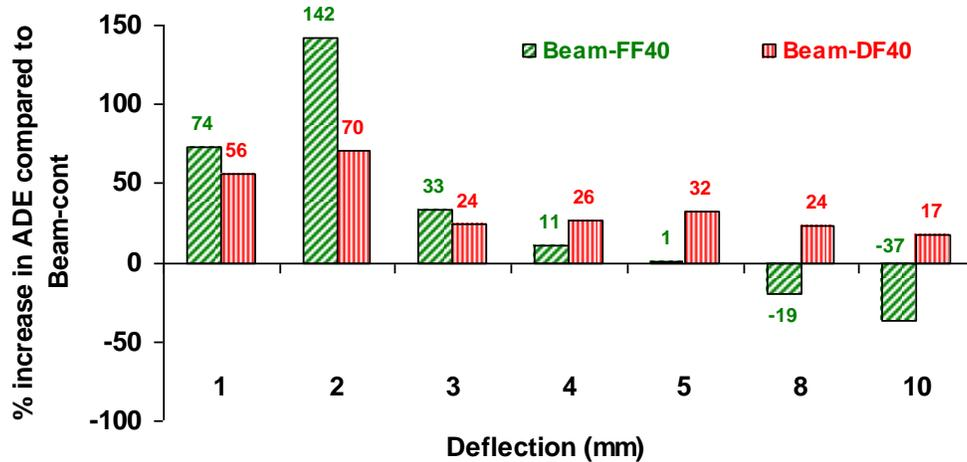
**Figure 10:** Percentage increase in ADE by the RC beams with fibers compared to Beam-cont
