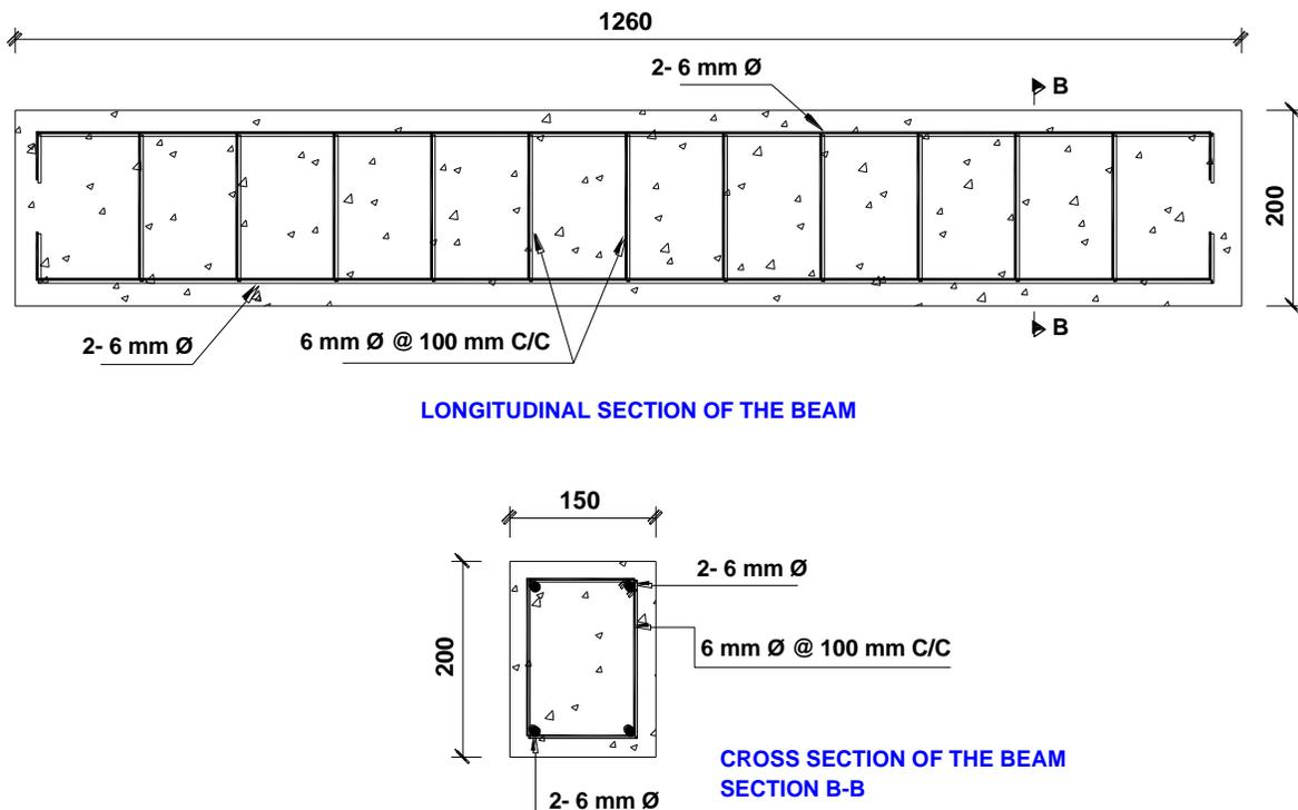
Figure 2: Reinforcement details of test specimen
