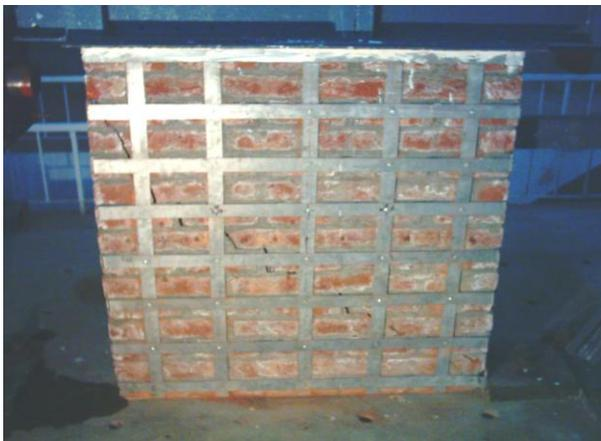
**Fig. 12** Shear failure of specimen FSM
