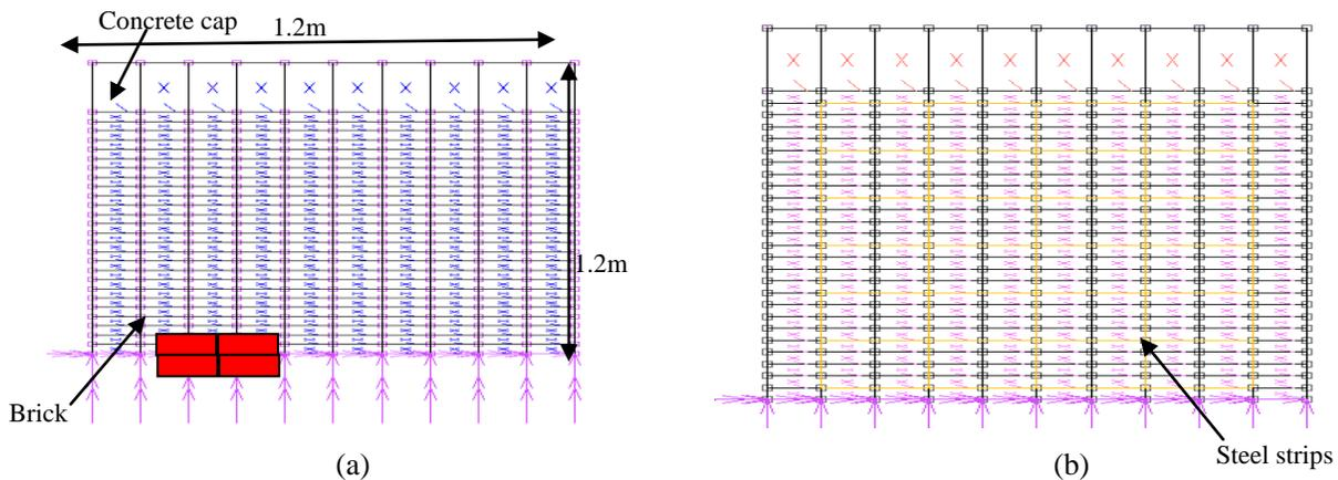
**Fig. 3** Geometric model of wall panels (a) un-reinforced masonry (b) strengthened masonry with fine steel mesh
