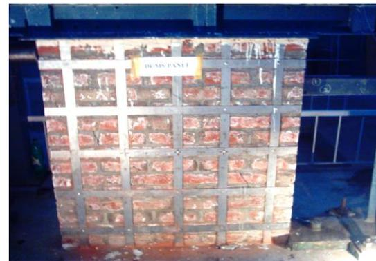
**Fig. 10** Shear failure of specimen SCM
