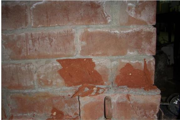
**Fig. 6** Sliding failure of specimen US
