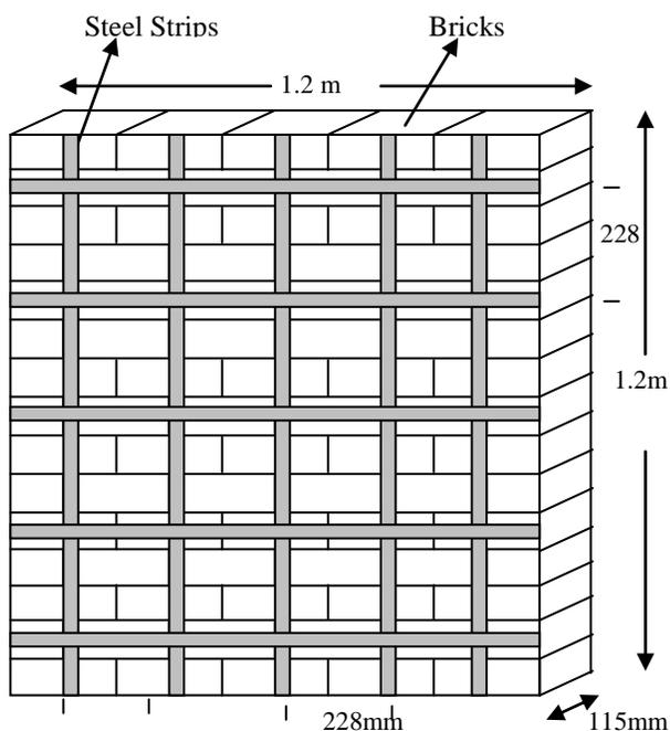
**Fig. 1** Line diagram of masonry wall panel
