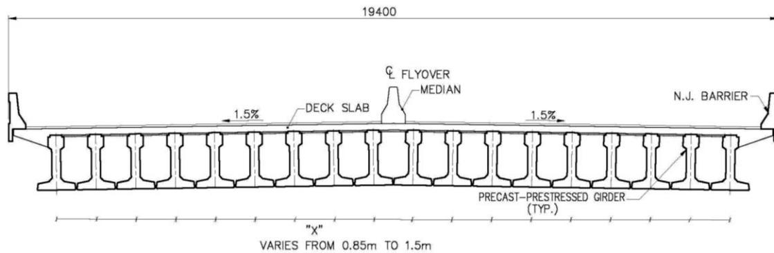
**Fig. 1** Bridge Cross Section for Inverted T Girder Super Structure
