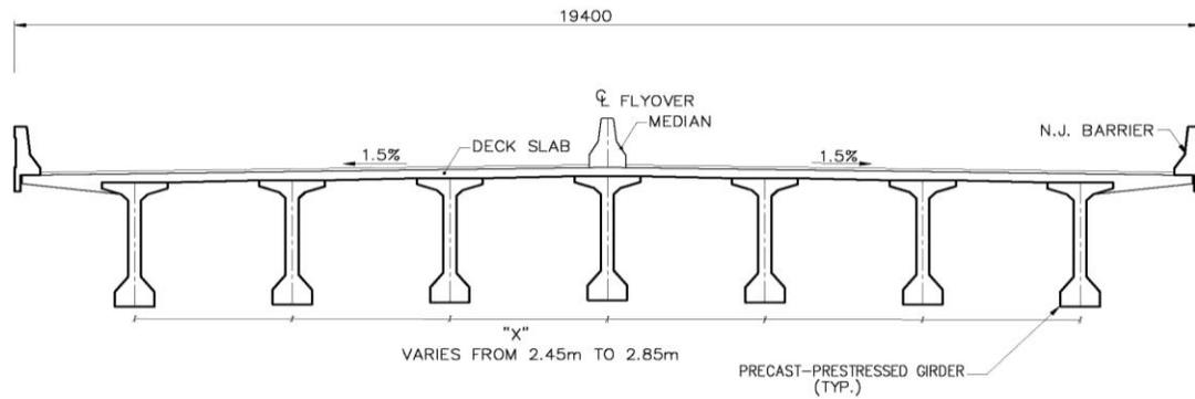
**Fig.3** Bridge Cross Section for NHA 'Type H' I-girder Super Structure
