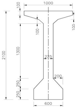
**Fig.4** Cross Section of NHA 'Type H' I-girder
