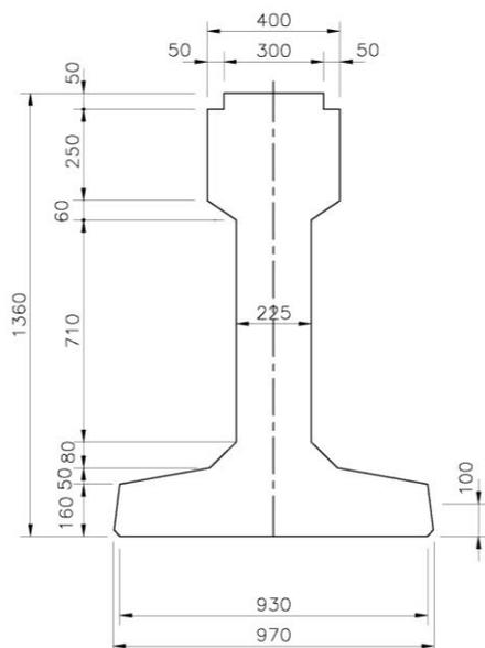
**Fig.2** Cross Section of Inverted T (IT) Girder
