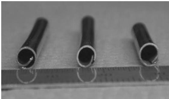
**Fig. 22:** Fe-SMA long twisted plates (Akikazu Sato et al., 2006)
