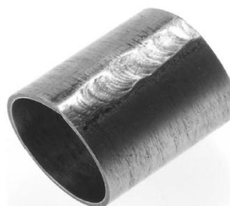
**Fig. 15:** Finished prototype Fe-SMA coupling (A. V. Druker et al., 2014)(A.V. Druker et al., 2015)
