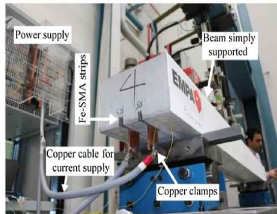
**Fig. 1:** Power supply to embedded Fe-SMA strips (Shahverdi, Czaderski, & Motavalli, 2016)
