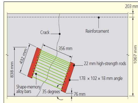
**Fig. 7:** Fe-SMAs rods crossing the cracks (Chang & Araki, 2016)
