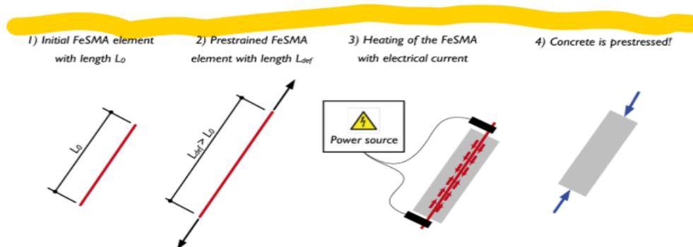
**Fig. 5:** Pre-stressing of concrete using Fe-SMA reinforcement
