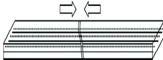
Fig. 10: SMA-wire contracts by electric heating and hence reduces crack (Mishra & Anish Ravindra, 2014)
