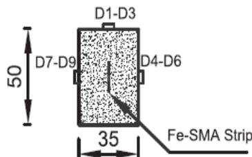
**Fig. 4:** Centrally reinforced Fe-SMA strip (Czaderski et al., 2014)
