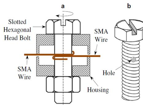
**Fig. 14:** Pre-strain ferrous FeNCATB SMA wires (F. Hedayati Dezfuli & Alam, 2014)
