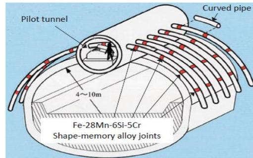
**Fig. 19:** Pipe joints of Fe-SMA (Sawaguchi et al., 2016)
