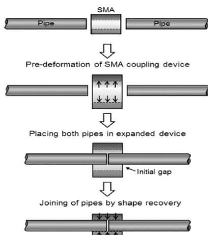
**Fig. 12:** Pipe Joining by using SMA Coupling (Lee et al., 2015)
