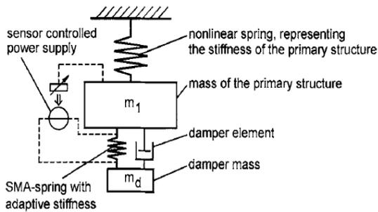
**Fig. 16b:** Fe-SMA-springs used in active vibration control (Janke, 2005)
