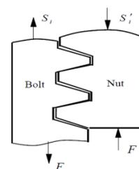
**Fig. 11:** Fe-SMA Nut (Junliang, DU, et al., 2015)
