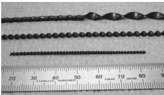
**Fig. 23:** Fe-SMA twisted wire (Akikazu Sato et al., 2006)
