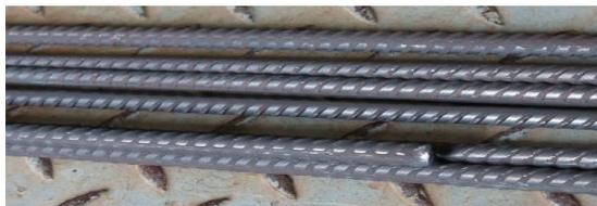
**Fig. 6:** 8mm Ribbed Fe-SMA bars used for concrete reinforcement
