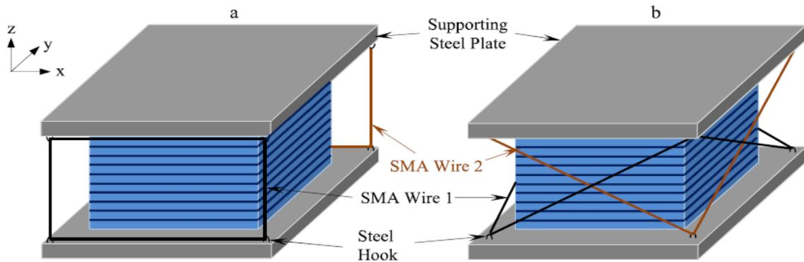
**Fig. 3:** Smart Rubber Bearings (a) straight SMA wires (b) cross SMA wires (Dezfuli & Alam, 2016; F. Hedayati Dezfuli & Alam, 2014; Farshad Hedayati Dezfuli & Alam, 2013)
