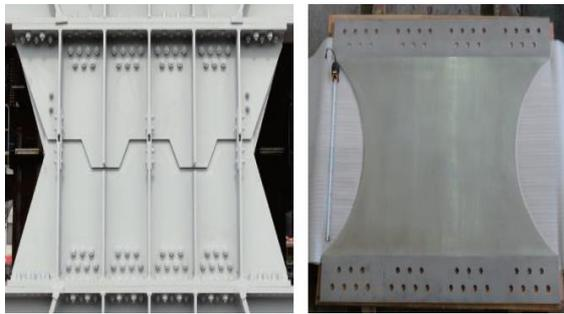
**Fig. 21:** Seismic Damper (Sawaguchi et al., 2016)
