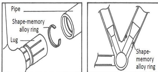
**Fig. 17:** Fe-SMA lock ring for frame pipe of a bicycle (Sawaguchi et al., 2016)
