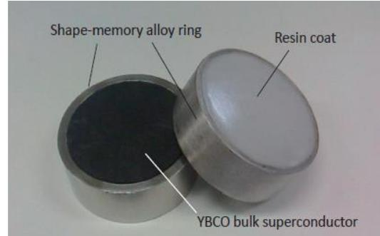
**Fig. 18:** SMA Ring to reinforce and protect bulk superconductor (Sawaguchi et al., 2016)
