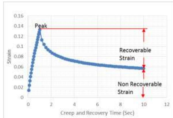
**Figure 3:** Result from 1 cycle of creep and recovery
