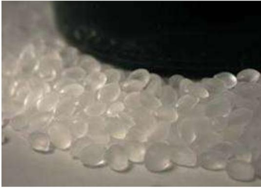
**Figure 1:** Elvaloy® RET polymer beads (Asphalt Mix Design Lab, Department of Transportation Engineering, U.E.T. Lahore)
